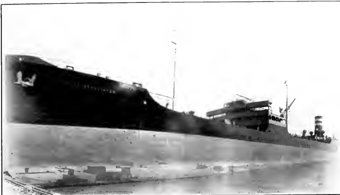
The newly completed motor tanker Tidewater Associated , equipped with Sun-Doxford opposed piston engines, tied up to the dock at the Sun Shipbuilding & Drydock Company where she was built.
